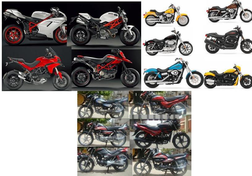
*Fig-5: Bikes from Ducati (left: Note the black, white and red color combination, high visual imbalance and trellis frame), Harley Davidson (Middle: Note the bare construction, single surface fuel tank and large rake) and Hero Honda (right: Note the high value high chroma colors and high unity)*
