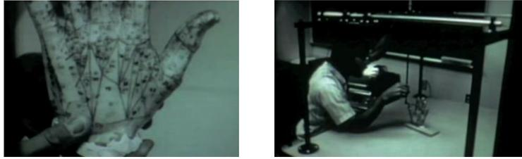
Figure 2. (a) Polygons drawn over a hand mock up for 3D registering of defining dots; (b) Digitalization of the hand with a 3D pointer which records all 3 coordinates.
