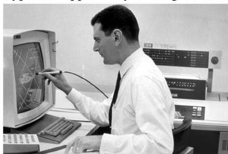
Figure 1. IBM 2250 Display connected to an IBM 1130 Computer
