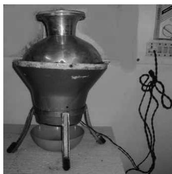
Figure 1. Innovator’s Functional prototype in of the pomegranate de-seeder
